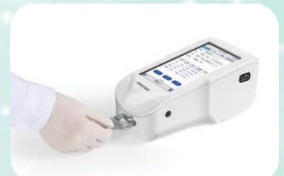
Step 3: Insert the cartridge into the analyzer until it clicks. Wait for the results
