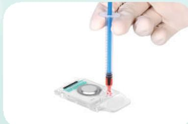
Step 2: Fill the inlet with sample to the fill mark and slide the cap to seal the inlet
