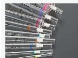
The pipet head is marked with different color codes, making the pipet range and model easy to identify
